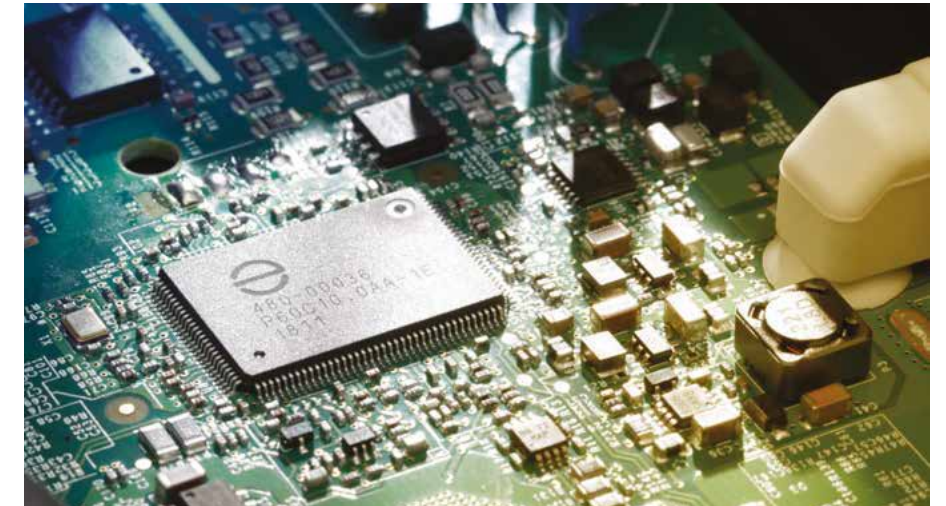
IQ 8 microinverter ASIC
